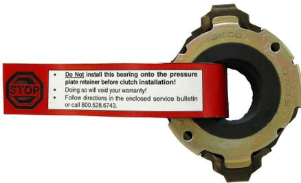
Most warranty on this kit involves improperly attaching the release bearing to the pressure plate diaphragm spring, even though we've included a technical bulletin (TB119) that explains the proper installation sequence of this unique bearing.
