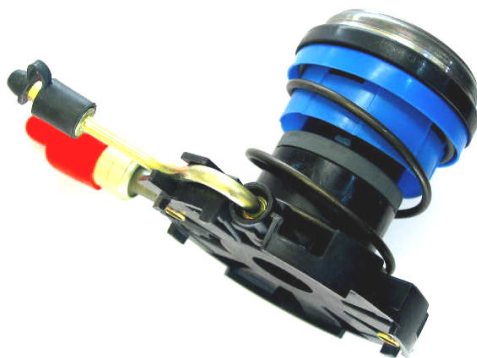
Early-style CSC without dust boot and revised release bearing
